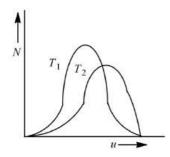
At both temperatures, distribution of molecules with increase in velocity first increases, reaches a maximum value and then decreases.
